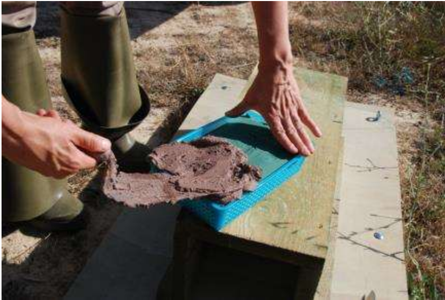
Figure 2. Mix of refractory clay and sand of approximately 0.5-1 cm, covering the sponge inside the basket. On this surface, the minks leave their paw prints.
