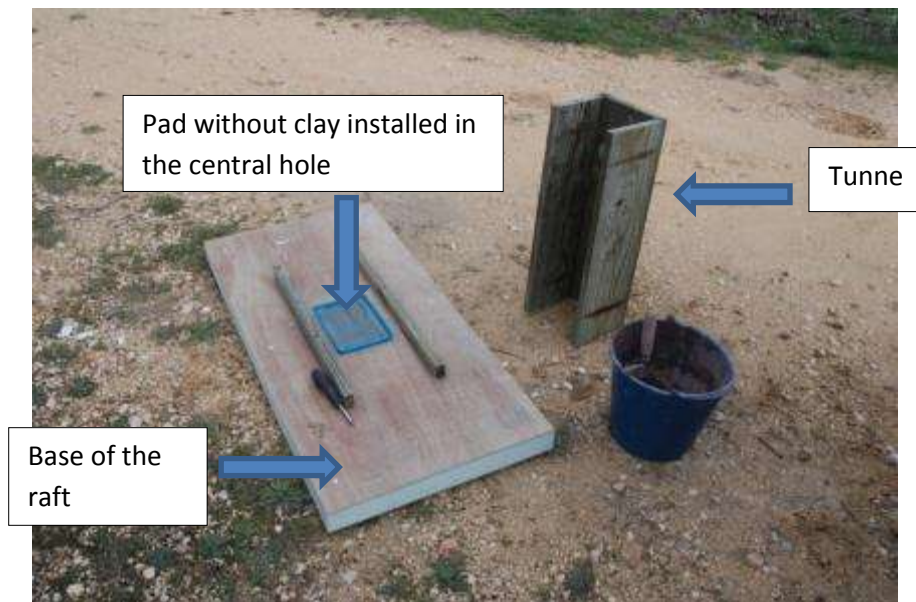
Figure 1. Mink raft before its final assembly (before placing the tunnel and covering sponge of the “pad” with the mix of refractory clay and sand).
